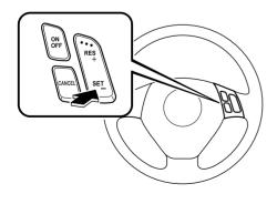
Your vehicle has a tap-down feature that allows you to decrease your current speed in decrements of 1.6 km/h (1 mph) by a momentary tap of the SET/- switch. Multiple taps will decrease your vehicle speed 1.6 km/h (1 mph) for each tap.
